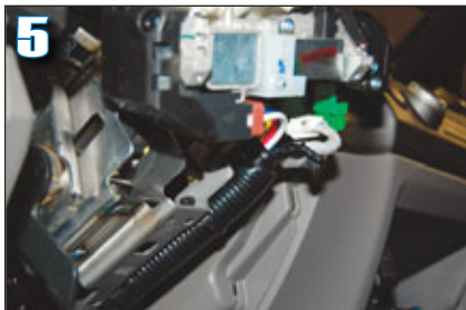
5 The transponder wiring is located at the steering assembly near the key cylinder.
