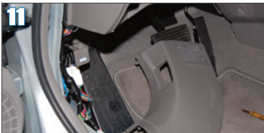
11 After the sill panel is removed, the kick panel pops off to allow access to the brake wire.
