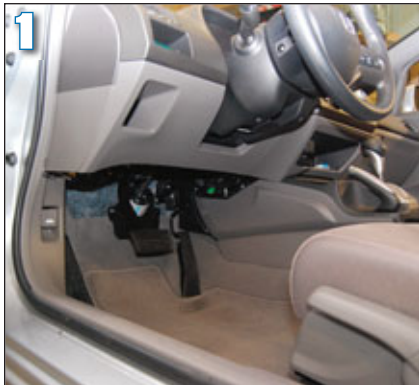
1 The steering column shroud and the panel below must be removed to gain access to the vehicle's wiring.
