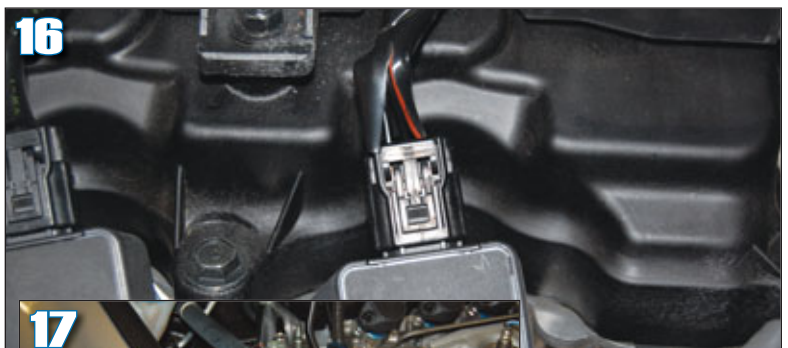
16 (Above) Close-up of the tach signal's location. (Left) The hood pin can be mounted on a bracket in the headlight area on the passenger's side.
