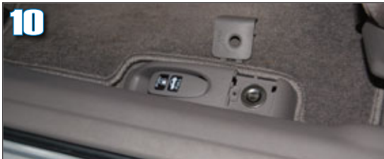
10 To remove the kick panel, the sill plate must be removed. The sill panel comes apart by popping the panel around the keyhole and removing one screw.
