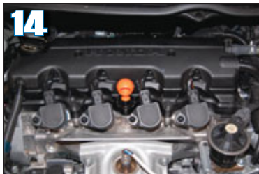
14 The tach signal is found underneath the "Honda" shroud that is held in place by two plastic fasteners. Each fastener requires a half turn to allow removal.
