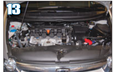
13 Find the tach signal in the Honda engine compartment.
