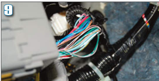
9 The lock-unlock wires are located behind the fuse box. The green wire is "lock," and the gray wire is "unlock."
