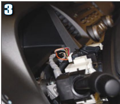
3 The horn wire is orange and located at the top of the steering wheel.
