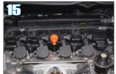
15 Now that the cover is removed, there is access to the vehicle's coil packs. Any wire that is not common to each pack can be used.
