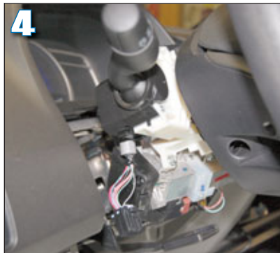
4 The negative parking light wire is gray and can be found under the wiper switch.
