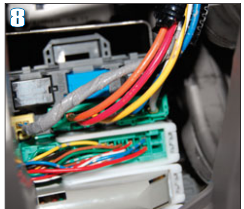
8 Constant 12-volt is the white wire. Ignition is the blue wire. Accessory is the orange wire. The starter is the yellow wire.
