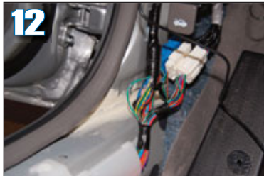
12 The brake wire is green and located in the driver's kick panel.
