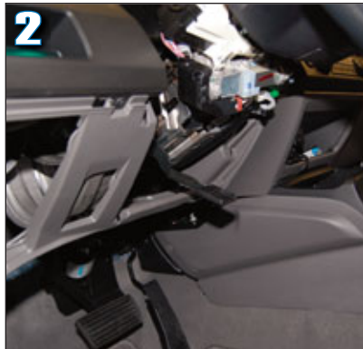
2 The under-dash panel pops off, and the steering wheel shroud is held in place with three screws.
